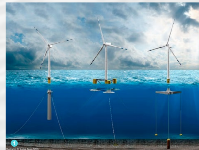
Figure 1 illustrates the three primary designs for floating offshore wind: tension leg platform, semi-submersible, and spar buoy. The semi-submersible and spar buoy structures, unlike the tension leg platform, are loosely moored to the seabed. This loose mooring configuration facilitates simpler installation processes. In contrast, the tension leg platform is firmly connected to the seabed.
